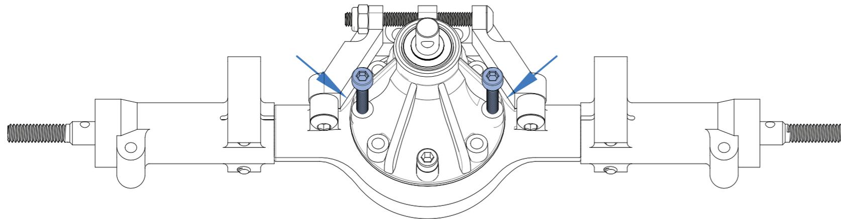
Step 3 - Lightly torque the screws until the third member is released
